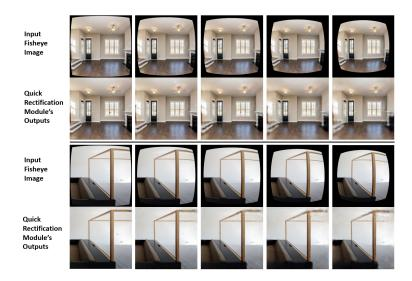
Figure 5: Our Quick Rectification Module demonstrates effective performance, rectifying curved structures back to straightened forms with high resolution.
