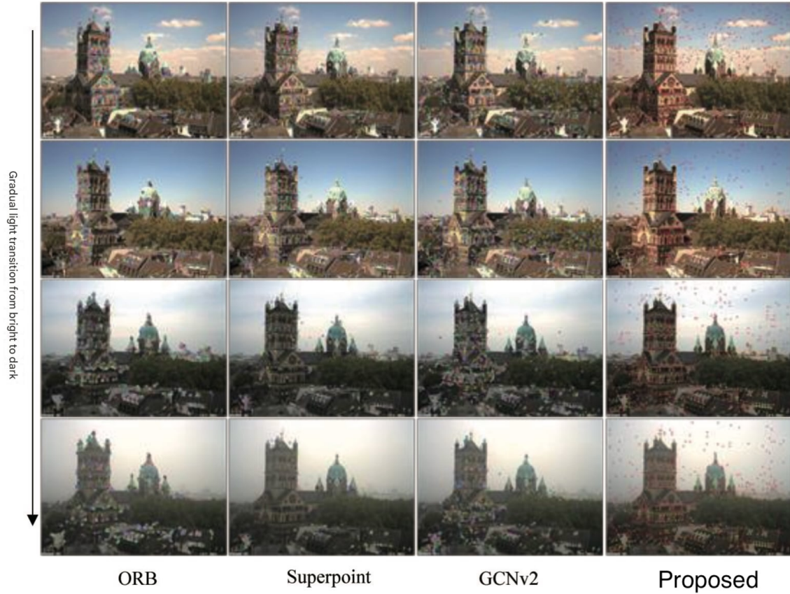
Figure 5: Detector responses on HPatches i_castle under illumination change. Top: input images; bottom: top- v detections (color encodes confidence). The position-prior detector preserves coverage and repeatability as brightness decreases.
