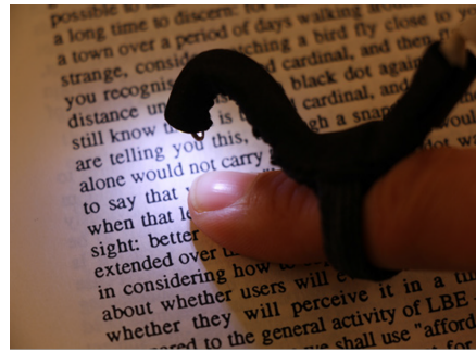
Figure 3: One of many HandSight prototypes which facilitates reading for the visually impaired.
