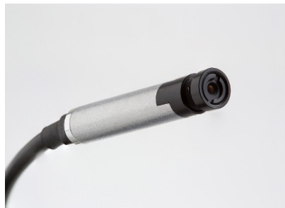
Figure 1: A NanEye GS camera - only a few millimeters in diameter.
