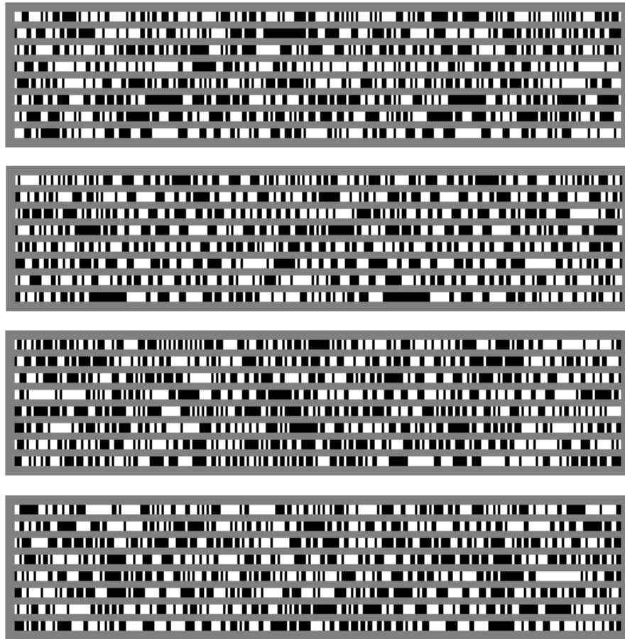
Figure 1: Representation of the IrisCodes [9], produced by four different eyes. The eight rows within each can be regarded as eight concentric rings, each encoding a [0, 2\pi] traversal around the iris. (Eyelid masking is not shown.)
