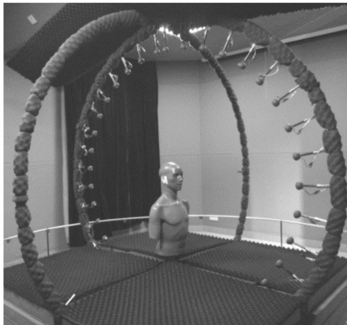
Figure 1: The schematic diagram showing the procedure for the measurement of HRTF [14].
